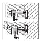
The shaft should be flush or under the surface of the rail end. Using a 5mm hex bit in a tool or allen wrench (fitted into the gear head), the shaft can be moved to engage into the disc keyhole. Then simply push rail downwards and tighten.
