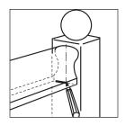
**3.** Mark final position of the hand rail onto post, observing the center line.
