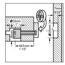
**4.** Assemble the shaft and gear housing into the rail.
