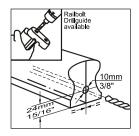
Mark position of 3/8" hole onto end of rail. As an alternative to marking hand rails for drilling, the Railbolt Drill Guide is available, making it fast and easy.
