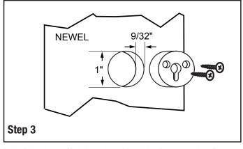
Drill 1" dia. hole 9/32" deep. Install keyhole disc so that it is flush or slightly under the post. Secure disc with screws. (Tip: Pre-drill holes to accept screws)
