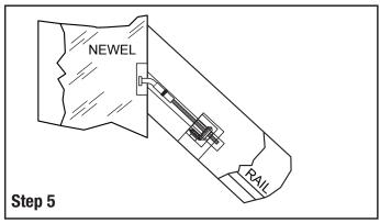
When proper fit is complete, glue and insert angled tip and tighten into place with 5mm driver and ratchet or allen wrench. Glue and insert a wooden 1" dia. plug. Sand flush with bottom of rail.
