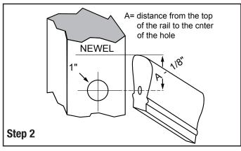
Cut rail at pitch from 1/8" mark. Measure distance from top of rail to center (A) of 3/8" hole on pitch (Note the measure). Now, mark a line on the newel that represents the top of pitch cut which is top of the rail. Then measure down the distance from top of rail to center of 3/8" hole (A), and subtract 1/8". This is the center of the disc.
