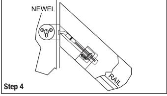
Slide rail on bolt and "dry fit" to be sure of proper angle and fit. If another cut is needed, take the least amount off to correct cut. The 3/8" deep hole that was drilled has allowed enough room for you to make this adjustment. Install bolt and gear head. Retract tip as far as you can to angle when sliding into position. You may have to exert a small amount of pressure on newel to help slide tip into position.
