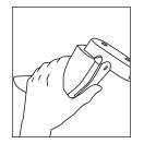
**Note:** The jig can also be used with an easement. Mark the center line and press firmly into end. Holding the end with one hand, align the flap, bending it to fit the easement. Align the holes through the windows in jig. Once lined up, the flap can be released and hole can be drilled. The "positioning pins" will help hold it in proper position to drill.
