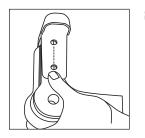
2. Be sure to align the jig with the "center line" by looking through the windows that are part of the jig. Once lined up perfectly using your hand, press the jig firmly into the end cut. It should fit flush against the end.
