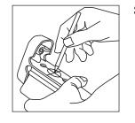
3. Using a pencil, mark the spot where the 1" hole on the bottom of rail will be drilled. IMPORTANT! Drill the 1" hole first before you drill the 3/8" hole. If not, it is possible that the bit will wobble and create an imperfect hole, and the 1" ZipBolt gear head will not fit properly.
