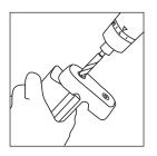
4. It is necessary to flip the jig during the process. The 1/4" hole is most commonly drilled into the fitting to accept the lag portion of the bolt. The 3/8" hole is usually drilled on the side where railbolt tightening takes place.
