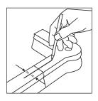
**1** Mark a "center line" about 3" long on each piece on the two sections being joined. In this case, it is a quarter turn fitting and a section of straight rail.
